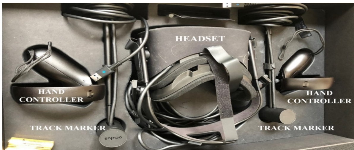
Figure A2 Oculus Rift VR devices consist of headsets, hand controllers, and track markers
