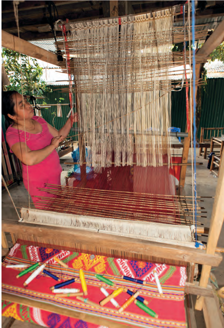
Figure 16. Weaver in the Mai Chau area, using a modified circular drawloom heddle (C3 type). Instead of using the warp lifts from the heddle directly, Mai Chau weavers use them to insert a set of pattern sticks in the warp (visible below the heddle system). The weaver then sits back down by the cloth beam and uses the sticks in the warp to insert wefts, removing each stick as she does so.
