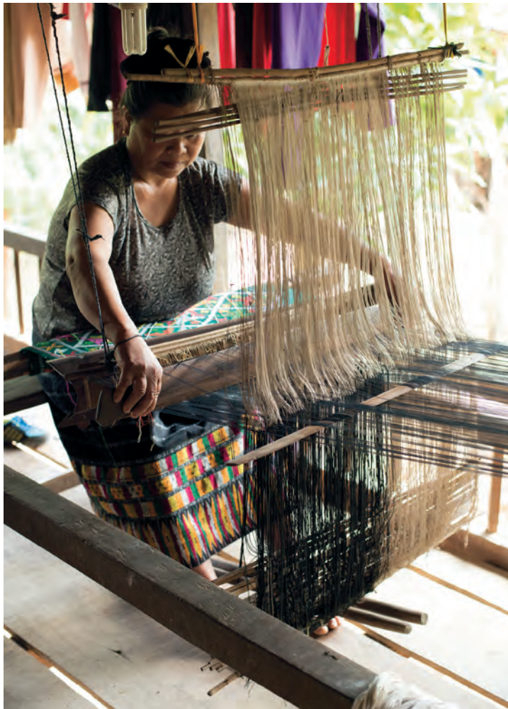
Figure 14. Weaver in the Ky Son area, northern Vietnam, using a VB type drawloom heddle to make a skirt cloth patterned with supplementary weft designs.
