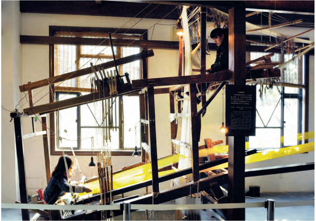
Figure 23. Working drawloom at the Suzhou Silk Museum, China. The weaver (at left) inserts the weft and works a set of treadles (shafts) that produce groundweave and satin effects. The drawperson (at top right) manipulates the pattern harness, which consists of pattern cords embedded in loops that connect with leashes. The lifts are transmitted to the warp via the set of vertical leashes below the drawperson. In some loom setups one pattern loop may connect with several leashes, making pattern repeats along the weft direction.
