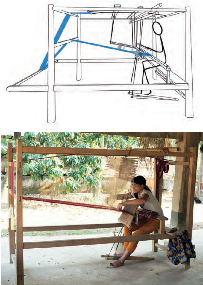
Figure 11. Full-frame loom, cuboidal type. Above: drawing of a loom used by a Tai Lao weaver in Vientiane, set up to weave a supplementary weft skirt hem, using a series of individual pattern heddles suspended above the warp. Below: a weaver in the Quan Son district of northern Vietnam, using a similar loom with a V-shaped pattern system.
