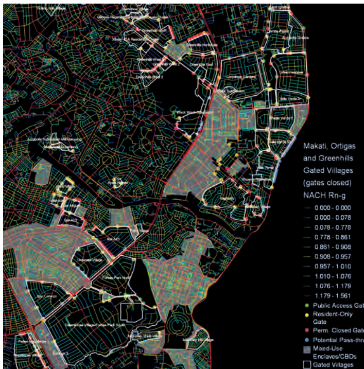
Figure 28. 2019 Spatial graph of Makati, Ortigas, and Greenhills Enclaves, showing Global Integration Centralities under the Gates Closed/Status Quo condition. This represents how access gates suppress the generative capacity of the spatial network within the villages; drawn by author using OpenStreetMap.
