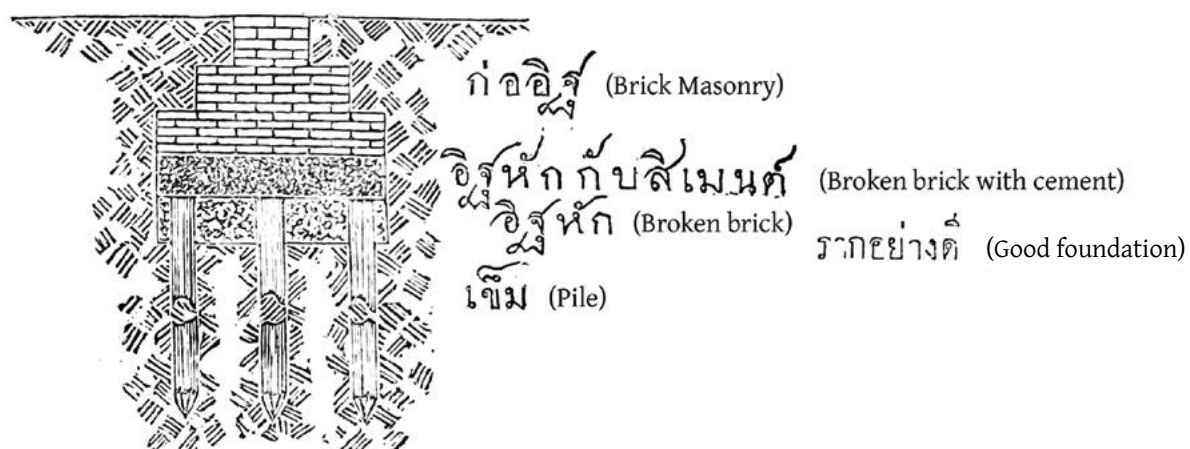
FIGURE 1: A diagram of a foundation considered the most effective and recommended for constructing a stable foundation in 1909 © Ploy & Ju 1909: I, 17
