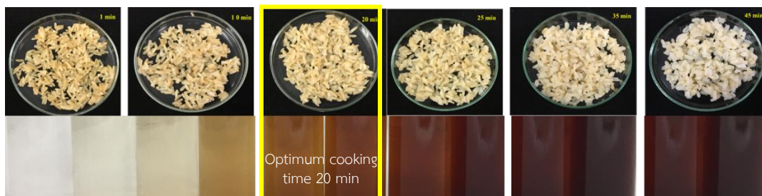
Figure 5 Relationship of rice cooking and TTI color changing 100°C.
