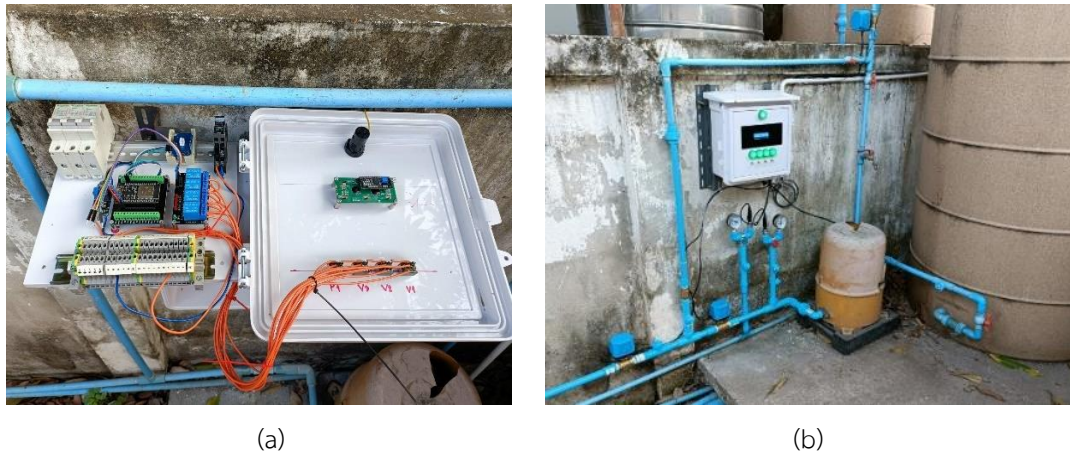
Figure 4 Overview of the proposed system (a) Control devices and circuitry, (b) Practical installation in a residential
