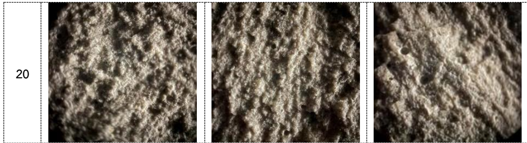
Figure 10. Image of cement composite material blended with RCA (50x)
